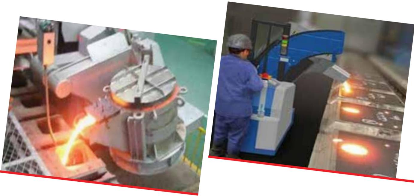
**Future:** Advancement in technology has led to the development of pressurized pouring furnaces which have a bottom pouring system and regardless of the level of molten metal, it always provides constant flow rate. It uses vision technology to regulate flow rate and positioning, which results in an efficient pouring technique.
